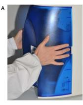
• Open the front cover of the system (A). This will allow the system to go into STANDBY mode once the system is powered.
