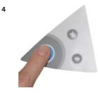
To exit the menu, press and hold the Main Button for 2 seconds.
