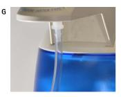
Install the Barbed Fitting and Tygon Tubing (G). (See Section Installation of the Tygon®Tubing).
