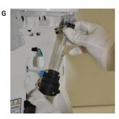
• Ensure that you use the gloves supplied with the UV replacement kit. Plug the electrical cable to the new UV Lamp (G).
