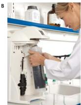
• Install the SimpliPak until it is fully seated into the system ports as shown (B, C and D).
