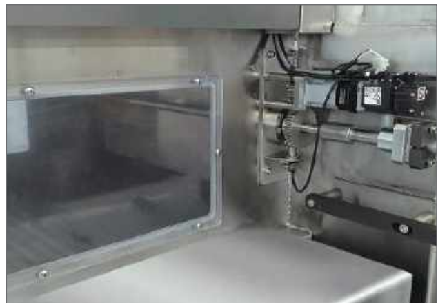
Auto Damper device(Servo motor applied)
