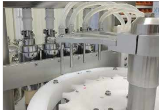
Filling Pump & Nozzle
